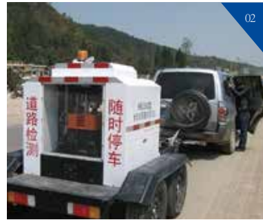
2-HBL550型拖车式落锤弯沉仪
